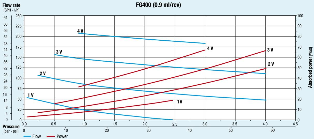
Note: Characteristics with water at 20 °C (68 F) and without relief valve. Fluids different from water must be validated by the Customer. Temperature requirements different from ambient temperature must be mentioned on the order. Different materials are available upon request. Use a filter before the pump inlet no larger than 10 micron
